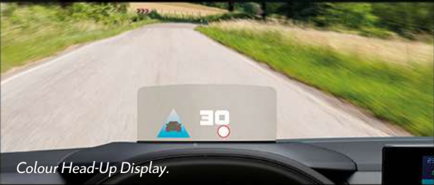
Colour Head-Up Display. The Colour Head-Up Display allows the driver to keep their eyes on the road while having the key driving information in their field of vision.
