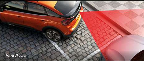
Park Assist. Park Assist detects a space, then operates the steering to park. The driver just needs to engage reverse gear, accelerate and brake.
